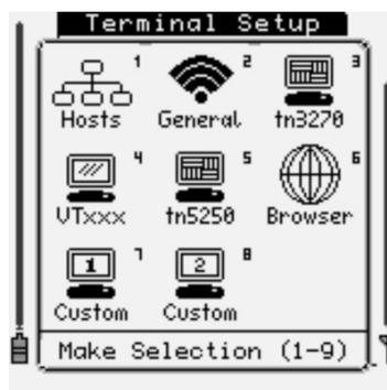
The Triton comes standard with VT100/VT220 interpreters, TN5250/3270 emulators, a standards compliant web browser, and supported SSH client. Any of these applications/emulators can be used to connect to remote network servers through the Connect / Reconnect menu. From here in the Terminal Options menu, this connection menu can be set up.
