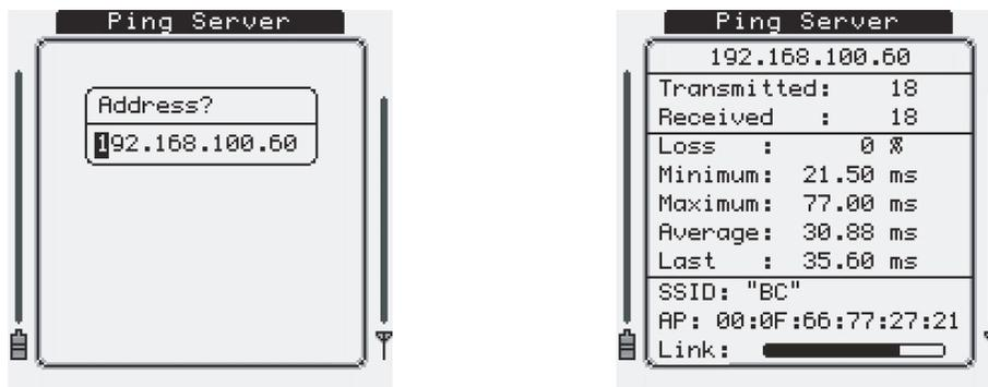
The Ping Server function allows testing of the active wireless network connection.
