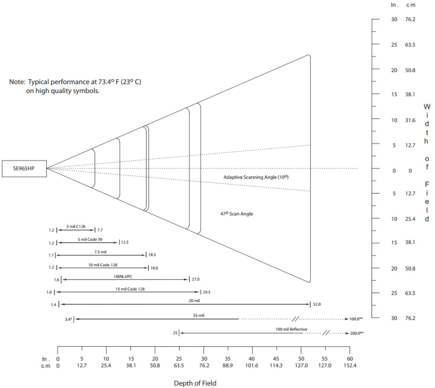
Reading distance for the Standard High Speed Laser
