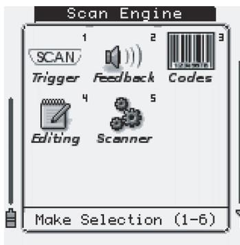
The Scanner Options group contains all aspects of the bar code decoder and data capture device. Within this menu are five sub groups: Trigger, Feedback, Codes (Symbologies), Editing, and General Setup.
