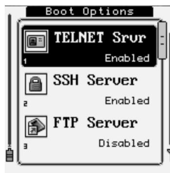
The Startup options give control over system services and servers that will be started on boot. They include a standard TELNET server, SSH / SFTP server, FTP server, embedded HTTP server, the bar code scanner manager, and an alternative 'Text Mode' menu navigational system.
