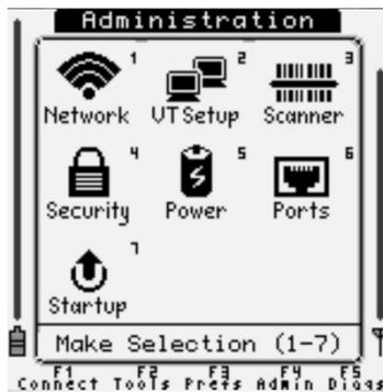
The Triton Administration menu houses all of the system's operating parameters, and from this menu, the entire system can be modified for use. Since the Triton contains hundreds of customizable options, each parameter is categorized into one of nine major groups, and some into smaller sub-sections. This allows each setting to be modified in a quickly and easily. The nine major settings groups are:
