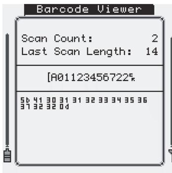
The Barcode Data Viewer displays the data acquired by the bar code scanner, including non-printable characters. The display shows both the printed values, as well as the hex encoded ASCII. Press [Esc] to exit the Viewer.
