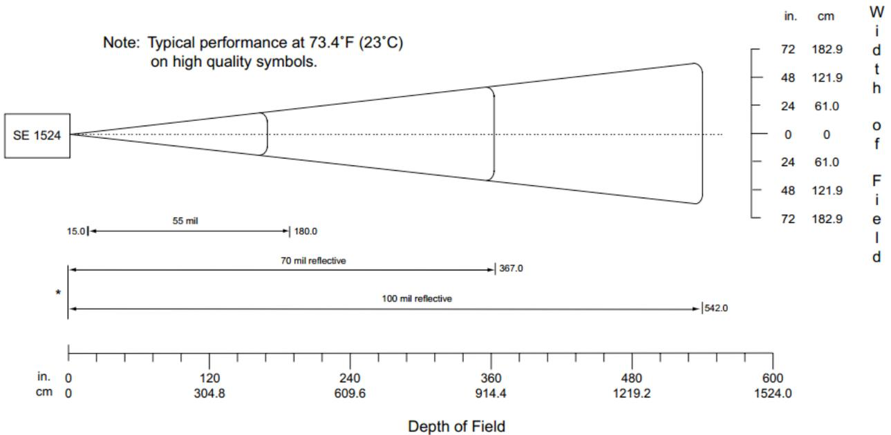
**Reading distance for the Lorax (SE1524) Laser**
