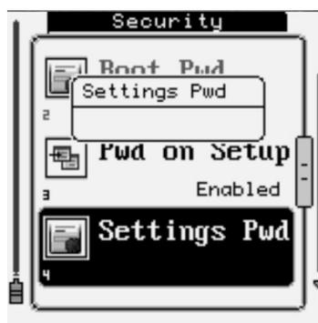
The Settings Password, if enabled, requires the user to enter a password to authorize changes in the settings. It is always a good idea to enable a Settings Password to prevent users from altering the unit's settings.
