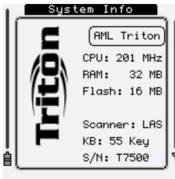
The Triton System Information screen shows data about the hand-held computer's hardware, including the CPU clock speed, installed scan engine, keyboard type, and the unit's serial number.
