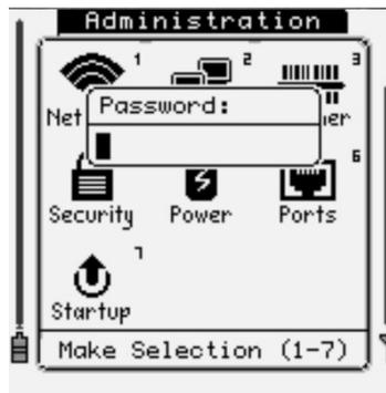
*\*NOTE: If a Settings Password is set, the Triton's embedded website password will also be changed to this password. If no Settings Password is set, then the embedded website password defaults to 'aml'.*
