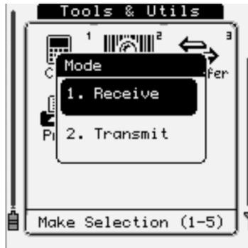
The Transfer applet allow the user to transmit the Triton settings files to a PC. Make sure that at least one port in the Port Settings menu is set to "Data Uplink" before attempting to transmit.
