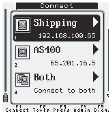
When the Triton first powers up, the unit will automatically attempt to connect to the host server. If more than one host connection is configured, the user will be prompted with the Connect menu, allowing them to select the server to connect to. If exactly two host connections have been configured, the "Connect to Both" option will be available.
