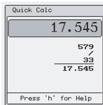
The Triton contains a simple, easy to use calculator. It can do simple mathematical functions by simply typing data from the keypad. Press [Menu] to return to the Triton menu system.
