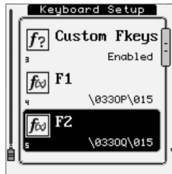
The keyboard setup menu allows you to streamline manual input and globally customize the function keys on the keyboard. These settings effect the actual Linux kernel keyboard mapping, allowing for complete control over these keys. See the Keyboard Option Parameters table for more information on customizing these keys.
