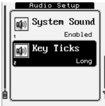
The audio setup menu is used to adjust system audio feedback. You can enable/disable all system sounds or adjust audible key tick feedback (short, long, or disabled).
