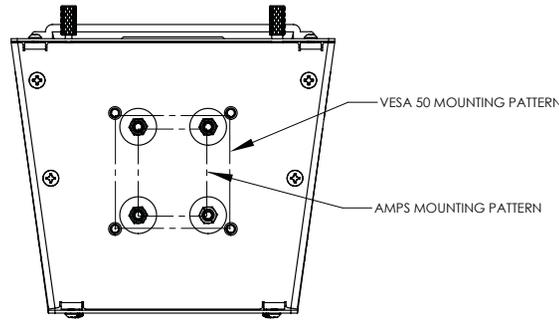
Device can be mounted using anti-vibration rubber mounting and mounting hardware.
