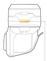
Plug the cable from the power supply into the USB-C connector on the rear of the device.
