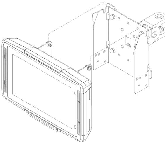
RE-INSTALL THE 2 BOTTOM BRACKET SCREWS.
