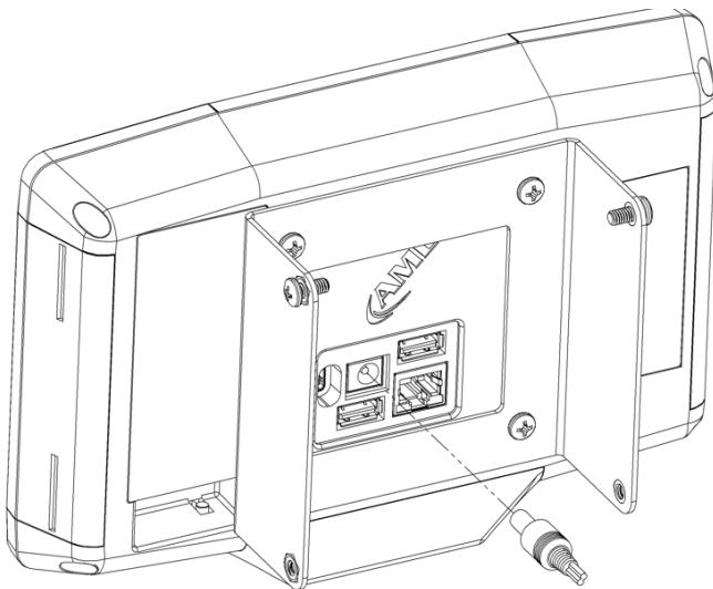
SECURE BRACKET REAR PANEL TO THE DESIRED MOUNT
