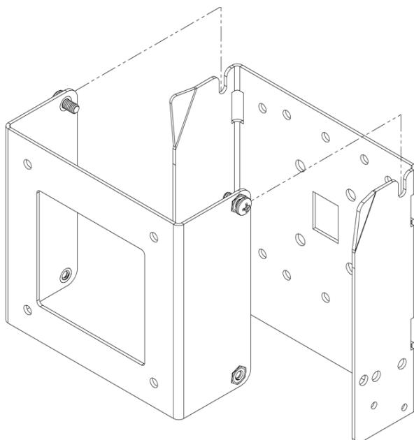
SECURE BRACKET FRONT PANEL TO DEVICE USING THE M4 SCREWS PROVIDED WITH THE DEVICE.
