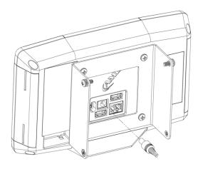
WIRE THE DC CABLE PROVIDED WITH CONVERTER KIT TO THE +VOUT (RED WIRE)
