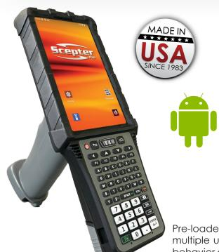
Scepter Pro sets a new standard in mobile computing with an impressive 5.5" AMOLED display with 1080 x 1920 resolution, producing vibrant colors and a sharp clarity not found on conventional TFT displays. The touchscreen display is optically bonded with Gorilla® Glass and features a NIT brightness rating of 500, suitable for indoor and outdoor visibility. The ultra-high resolution and superior contrast ratio makes even the smallest text well defined and legible.
