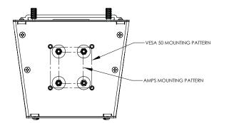
Device can be mounted using anti-vibration rubber mounting and mounting hardware.
